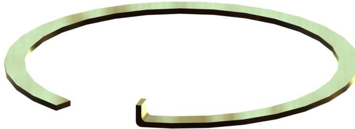
The bent end offers a "nose" which hinders the rotation. No additional keystone needs to be handled in the assembly process. Time and costs for machining the additional groove is comparatively less.
