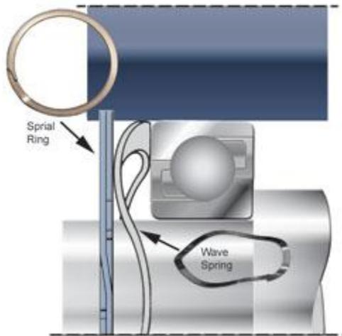
Alternatively, single-turn or two-turn wave rings can replace the retaining ring. These retain and pre-load the outer race of the bearing, streamlining the assembly process.
