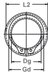
Clearance Diameter & Gaging Diameter Released in Groove.
