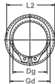
Clearance Diameter & Gaging Diameter Released in Groove.
