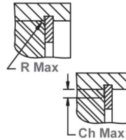
Allowable Corner Radius & Chamfer
